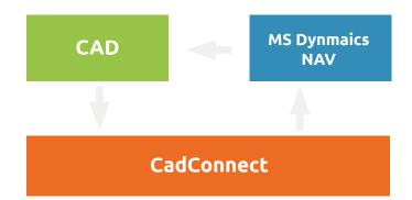
With CadConnect construction engineers can retrieve item numbers from MS Dynamics NAV, use the information for construction drawings — and export bill of materials to MS Dynamics NAV. Then routings and operations can be added to make it a complete production bill of material
